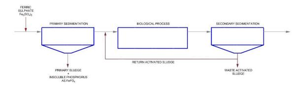
Pre-precipitation on its own is sufficient to meet an Orthophosphate ELV of > 0.7 mg/l.
