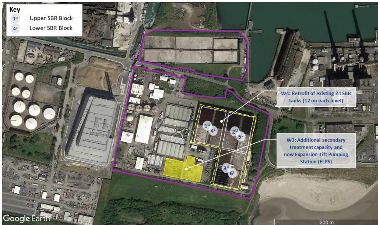
Figure 3-12: SBR tanks – Upper deck blocks 1, 2 and 3 and lower deck blocks 4, 5 and 6
