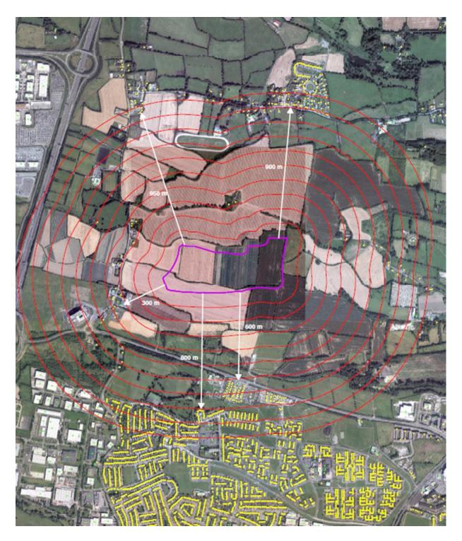
Figure 1: Distance from WwTP boundary to sensitive receptors
