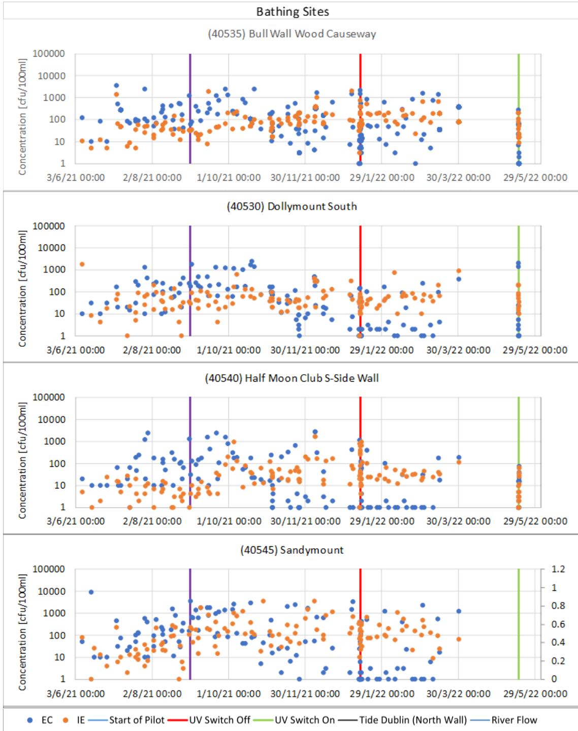
Figure 8. *E. Coli* and *Enterococci* Sample Data at selected bathing sites in close proximity to the Ringsend WwTP outfall.
