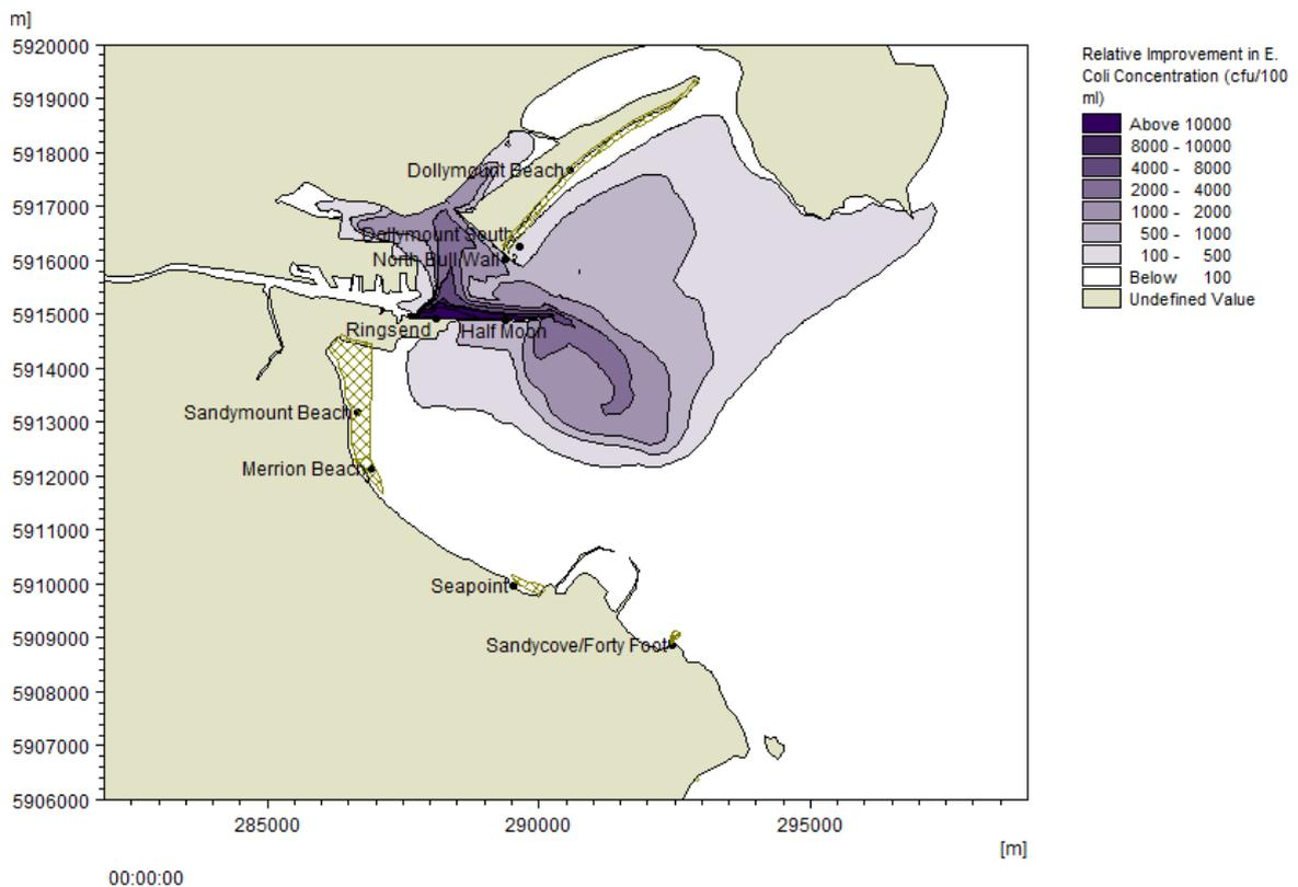
Figure 4. Modelled reduction in 95<sup>th</sup> percentile Winter E.Coli concentrations due to UV operation under calm, dry conditions.
