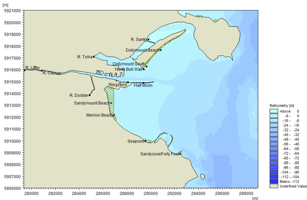
Figure 3. Model domain and bathymetry of the existing MIKE 3 Model of Dublin Bay
