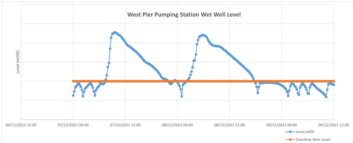
Figure 15. West Pier Pumping Station Wet Well levels
