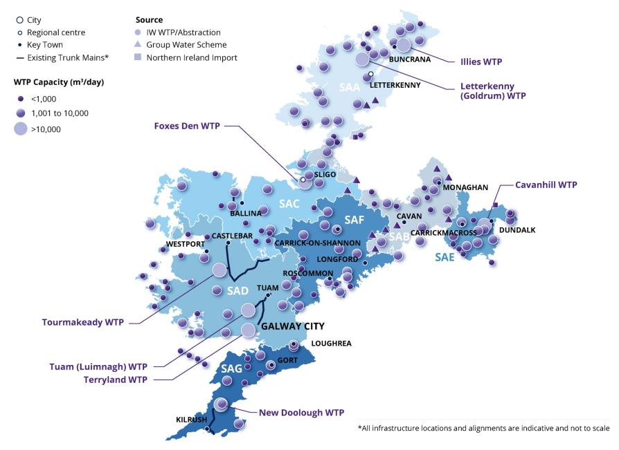
Figure 10.1 Existing Water Treatment Plants (WTPs) and Major Interconnecting Pipelines (Trunk Mains)
