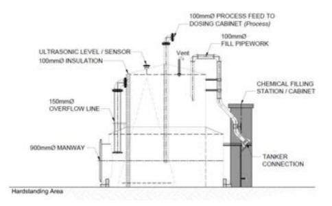
Figure 2 Sectional view of typical circular free standing chemical storage tank.
