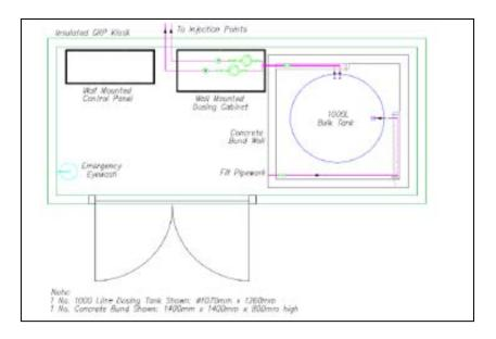
Figure 3 schematic of a bulk tank kiosk layout in H³PO<sup>4</sup> Installation with 500 litres< bulk storage ≤ 6,000 litres.
