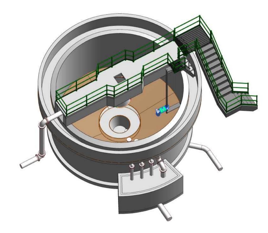
3D View - Sludge Thickening Tank Copyright
