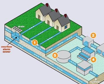
float to the surface. The settled and floating materials are removed and the remaining liquid may be discharged or subjected to further secondary treatment.
