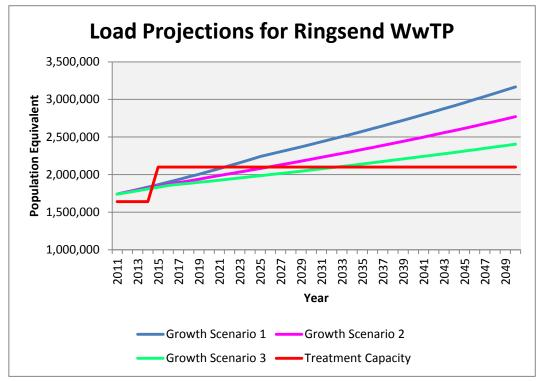
Fig. 4.1 Loading Projections for Ringsend WwTP.
