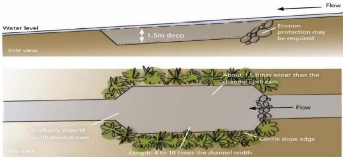
Figure 3. Cross-section and plan views of a sediment trap (Source: [https://www.dairynz.co.nz/media/254172/5-9 sediment traps 2012.pdf](https://www.dairynz.co.nz/media/254172/5-9_sediment_traps_2012.pdf))
