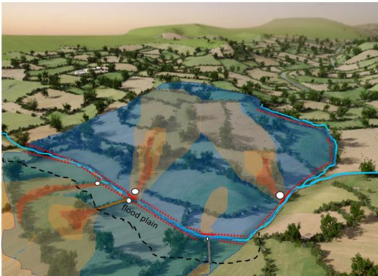
Figure A2: Illustration of a phosphate critical source area (CSA), flow delivery points, flow delivery paths, focussed flow delivery zones and dispersed flow delivery zones. (Produced in consultation with Eva Mockler, Catchments Unit, EPA.)
