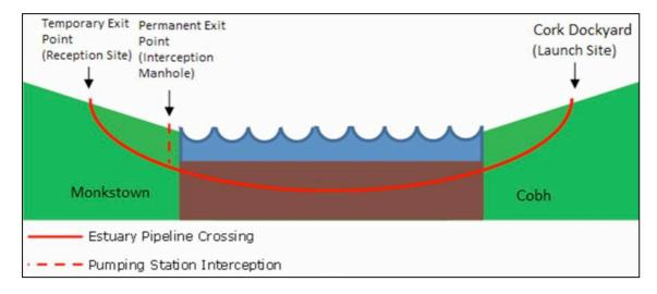
Figure 3 Schematic showing section across estuary.
