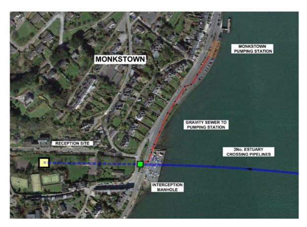
Figure 2 Proposed reception site and interception manhole with associated gravity sewer.
