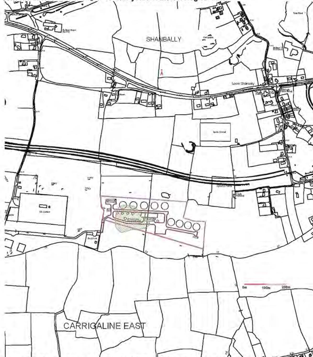
**Figure 8.3.** Predicted odour emission contribution of overall proposed Cork harbour WWTP to odour plume dispersal for grouped sources Odour control units 1, 2, 3, 4 and 5 for an odour concentration of less than or equal to  $0.30 \text{ Ou}_E \text{ m}^{-3}$  (—) at the 98<sup>th</sup> percentile of hourly averages for 5 years of meteorological data.
