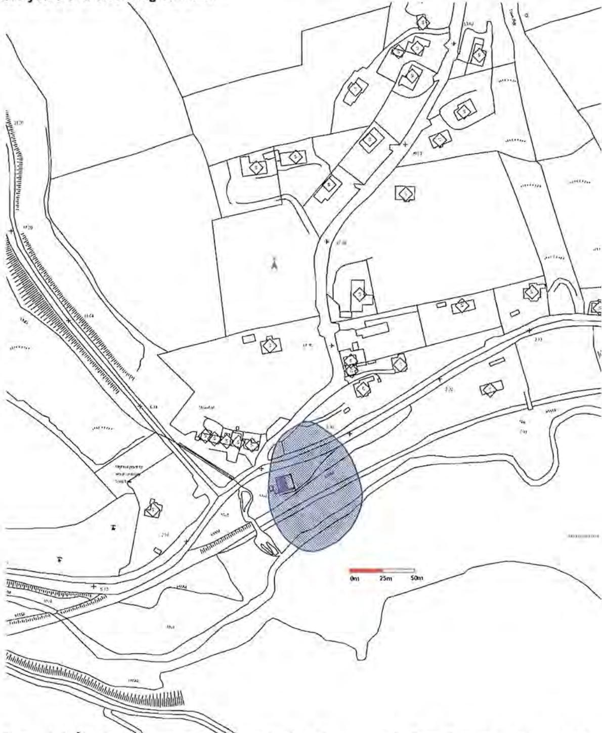
**8.6 Predicted odour emission contribution of proposed West beach Pumping station operation with odour abatement protocols implemented (ref Scenario 2) (see Table 4.2), to odour plume dispersal at the 98<sup>th</sup> percentile for an odour concentration of  $\leq 0.30 \text{ Ou}_E \text{ m}^{-3}$  for five years of meteorological data.**
