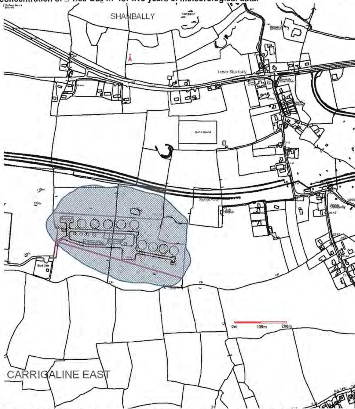
**Figure 8.1.** Predicted odour emission contribution of proposed overall Cork harbour WWTP operation with odour abatement protocols implemented to odour plume dispersal for Scenario 1 at the 98<sup>th</sup> percentile for odour concentrations  $\leq 1.5 \text{ Ou}_E \text{ m}^{-3}$  (—) for five years of meteorological data.
