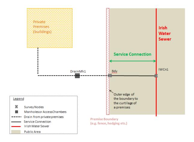
Figure 1 Typical arrangement of Drain, Service Connection and Irish Water Sewer
