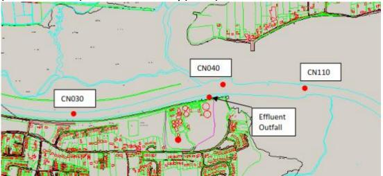
Figure 2: Location of the three transitional water sampling stations in the Castletown Estuary (CN030 and CB040) and Inner Dundalk Bay (CN110) in relation to the effluent outfall.
