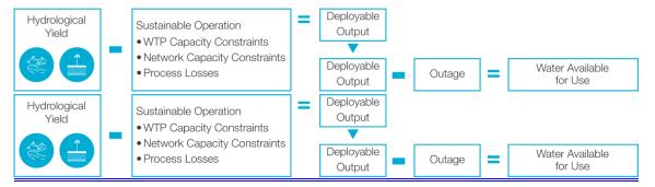
Figure 3.6 – WAFU Calculation Process
