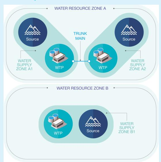
In this example, there are two WRZs and three WSZs. WRZ "A" contains two WSZs, which are connected by a trunk main. If there was an outage at the water treatment plant in WSZ A1, the area could continue to be supplied from the water treatment plant located in WSZ A2 (should sufficient spare capacity be available).
