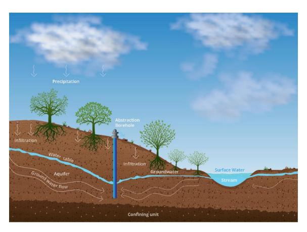
Figure 3.5 - Conceptual Model of a Groundwater Abstraction
