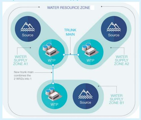
In this example there is one WRZ and three WSZs. A trunk main connects WSZs A1 and A2 with B1 to form a single WRZ. This arrangement offers greater resilience as, if there is an issue at the water treatment plant or with a source in WSZ B1, customer supply could be maintained from WSZ A1 or A2 (should spare capacity be available).
